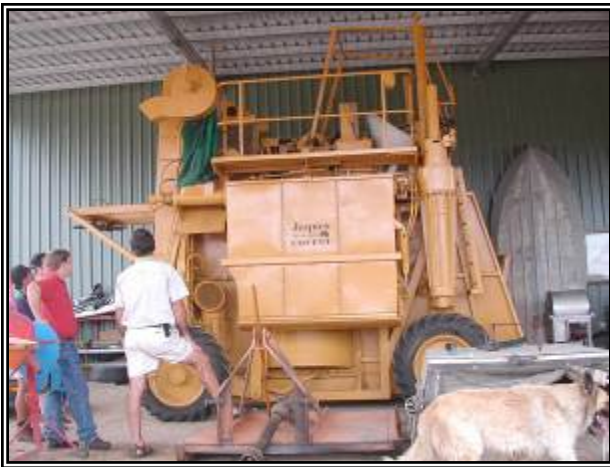
Nat Jaques shows his “Australians first coffee harvester”. Designed by him and his brother, built by NQEA shipyard.
