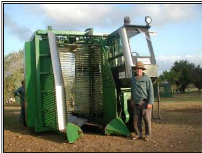
Noel Godfrey with his “Austoft” coffee harvester. Now called “Brastoft” and made in Brazil by Case.
