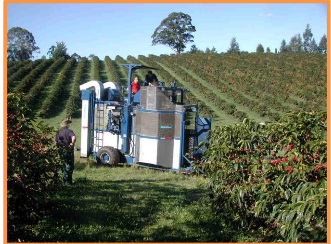
Mechanical coffee picking in Queensland Australia. Picking results 35% Over-Ripe, 55% Ripe, 10% Under-Ripe
